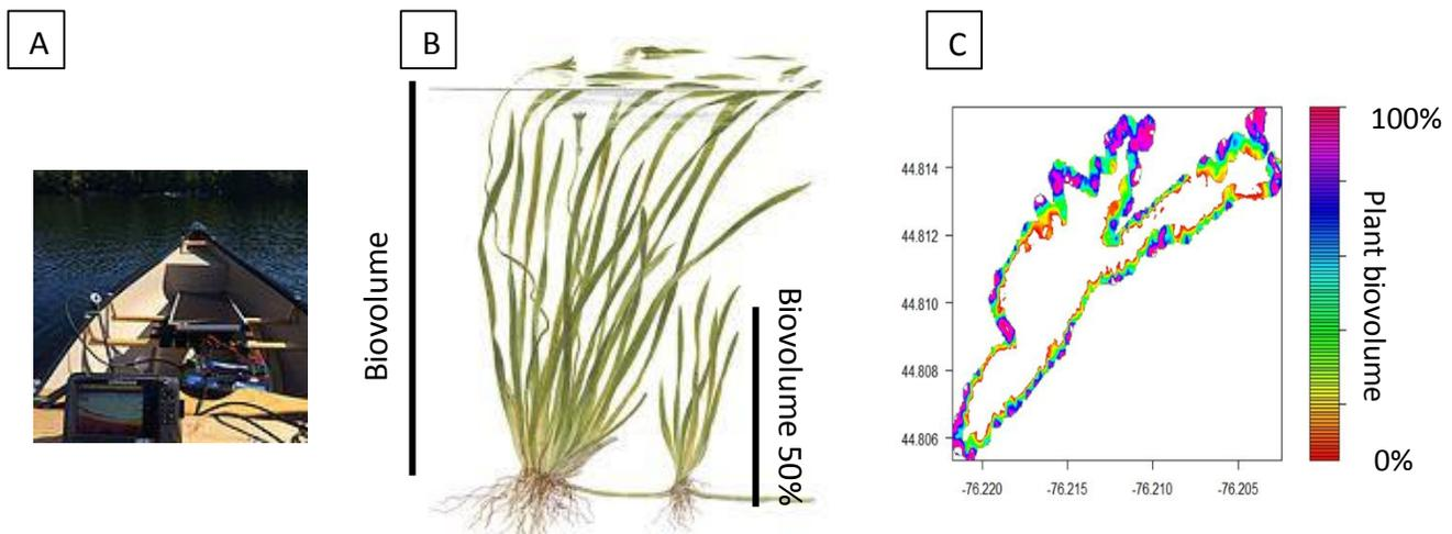
*Figure 6: A) Picture of a canoe outfitted with plant mapping echosounder. B) Example of plant biovolume at approximately 100% and 50% C) Example plant biovolume map from Adam Lake.*
